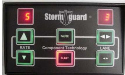
**Spreader Module in Blast Mode**
