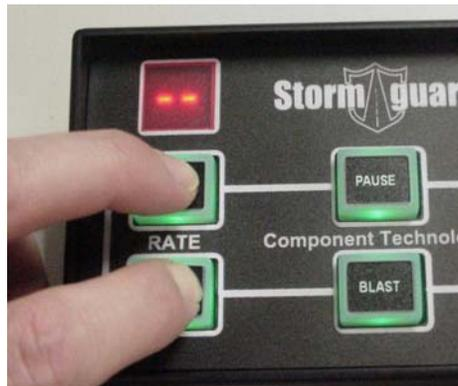
***To enter Setup Mode you must press both switches and hold them down until double dash is displayed on Rate Indicator.***
