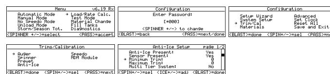
c) Shortcut: Minimum and maximum trim and pwm values can be entered manually by downloading the existing cal file and matching the pre-wet settings and AI settings. Upload new settings to the SS Rx.
