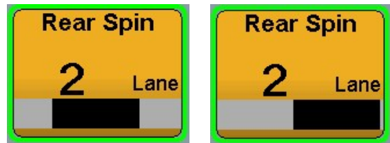
Figure 10: The image on the left shows the directional spinner centered. The image on the right shows the directional spinner angled almost completely to the right side of the truck.
