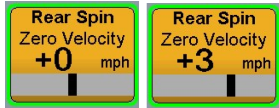
Figure 9: The image on the left shows the ZV spinner spreading at the road speed. The image on the right shows the ZV spinner is spreading 3 MPH greater than road speed.
