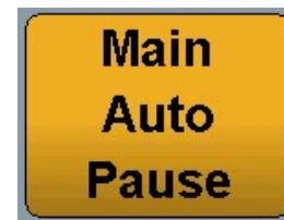
Figure 2: Spreader status showing the Main Spreader in "Auto" mode and in "Pause"
