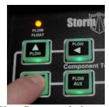
Push and hold Plow Down switch to engage Plow Float
