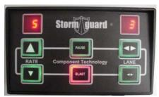
Spreader Module in Blast Mode
