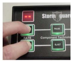
To enter Setup Mode you must press both switches and hold them down until double dash is displayed on Rate Indicator.
