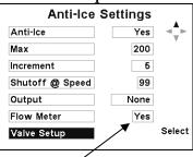
Note: Flow-meter is set to "YES". This is Closed-Loop operation.
