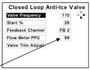
Enter directly: The flow-meter K-Factor or PPG (P)ulses (P)er (G)allon. Normally found on a Tag located on the flow-meter. PPG is always entered as US gallons in English or Metric modes of operation.
