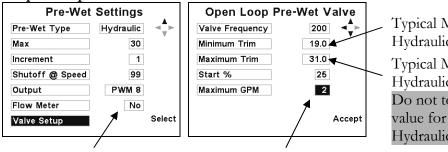
Typical Min Trim setting for a Hydraulic Stack-driven pre-wet. Typical Max Trim setting for a Hydraulic Stack-driven Pre-wet. Do not to exceed 40% max trim value for typical Hypro type Hydraulic motors.
