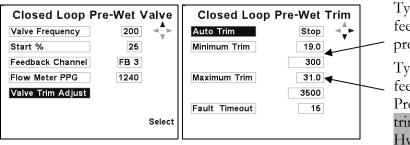
Typical Min Trim setting and pulses feedback For Hydraulic Stack-driven pre-wet.
