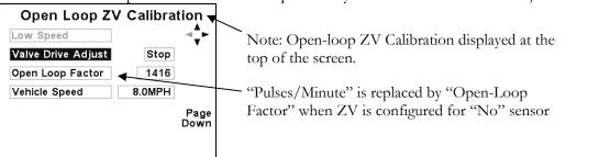
If calibrating a closed-loop system, open-loop values are automatically saved simultaneously while saving closed loop values. Open-loop values are necessary in event sensor failure occurs in operating closed-loop mode. The number value open-loop "Open loop Factor" is identical to the "Pulses/Minute" value for closed-loop systems.
