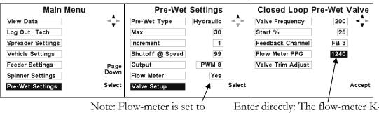
"YES". This is Closed-Loop operation. Enter directly: The flow-meter K-Factor. Normally found on a Tag located on the flow-meter. This is entered as (P)ulses (P)er (G)allons US even when in Metric mode.
