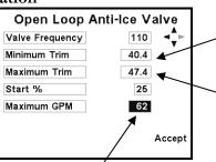
Adjust Min Trim until Pump is running slowly. Exit in and out of value to be sure pump starts reliably.
