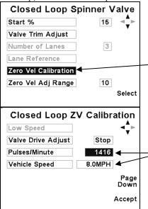
Select the Zero Vel Calibration menu to access calibration screen for "Low" and "High Speed" calibration points
