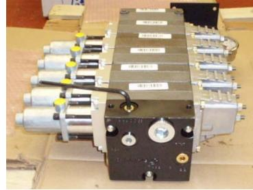
Using a 5/32" allen wrench, carefully install the 1/16" NPT cross drilling plug. Tighten till snug.
