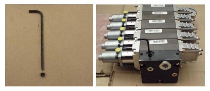
Re-install the -4 SAE port plug that was removed in step 1.
