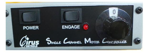
Power Switch: Main system power switch.
